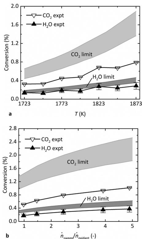
Fig. 4 Comparison of the average experimental conversion of CO<sub>2</sub> and H<sub>2</sub>O at steady state versus equilibrium limits as a function of (a)  $T$ , at  $\dot{n}_{\text{sweep}}/\dot{n}_{\text{oxidant}} = 2.4$  and 1 Pa O<sub>2</sub>, and (b)  $\dot{n}_{\text{sweep}}/\dot{n}_{\text{oxidant}}$ , at 1873 K and 0.5 Pa O<sub>2</sub>.
