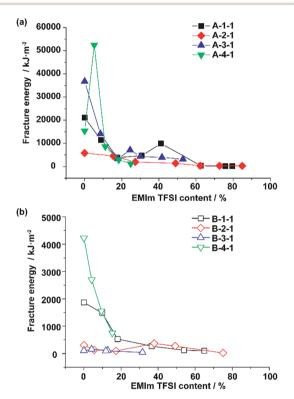
Fig. 2 Relationship between the fracture energy and ionic liquid (EMIm TFSI) content for (a) supramolecular ionic liquid elastomer (A-Acrylate-1) and (b) chemically cross-linked ionic liquid elastomer (B-Acrylate-1). [■: Methyl acrylate (1), ◆: ethyl acrylate (2), ▲: butyl acrylate (3), and ▼: methyl methacrylate (4)].
