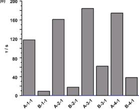
Fig. 3 (a) Stress relaxation behaviour of the supramolecular ionic liquid elastomer (A-Acrylate-1, solid lines) and chemically cross-linked ionic liquid elastomer (B-Acrylate-1, dashed lines) with a 5% strain for 1 hour. (b) Slow relaxation time constant of the A-Acrylate-1 and B-Acrylate-1. Acrylate: methyl acrylate (1), ethyl acrylate (2), butyl acrylate (3), and methyl methacrylate (4).
