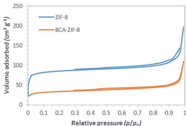
Fig. 4 The N<sub>2</sub> adsorption isotherms of ZIF-8 and BCA-ZIF-8 at 77 K.
