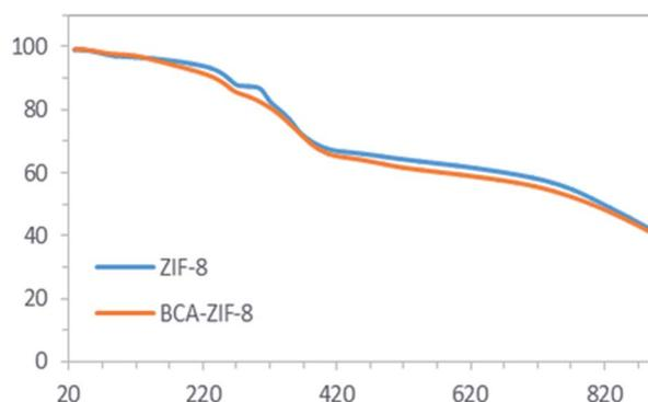
Fig. 5 The TGA curves of ZIF-8 and the BCA-ZIF-8 composite.
