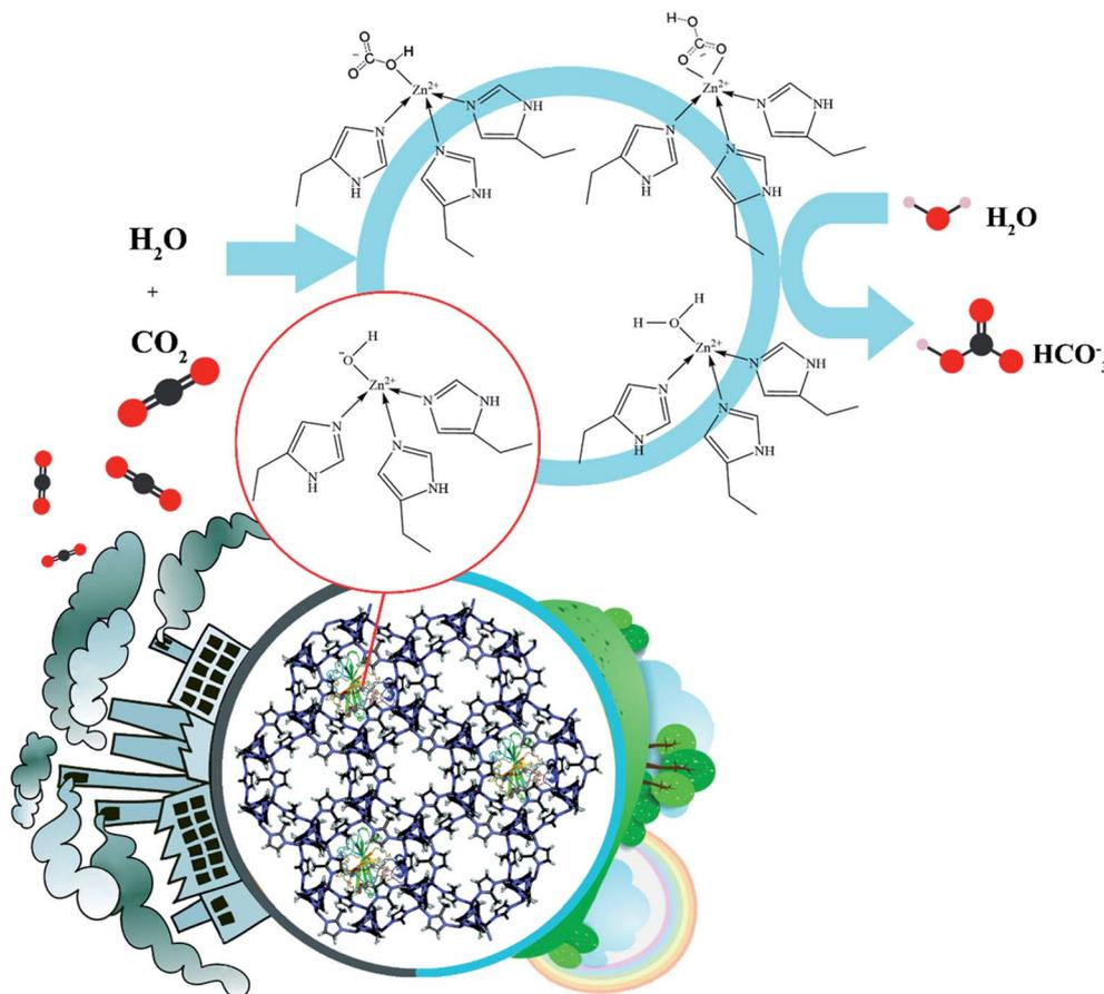
Scheme 1 Utilization of BCA-ZIF-8 biocomposite in the biocatalytic hydration of CO<sub>2</sub>.
