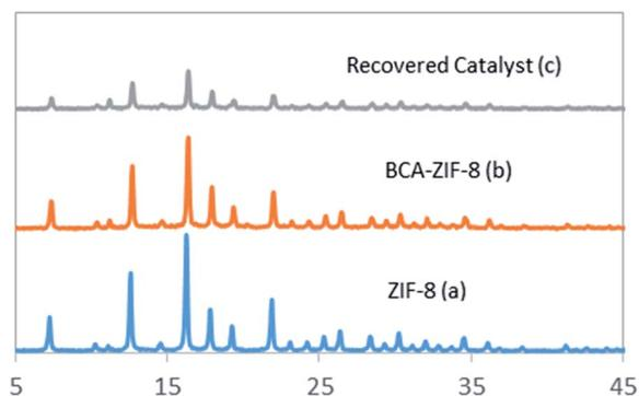
Fig. 1 The PXRD patterns of ZIF-8 (a), BCA-ZIF-8 (b) and recovered BCA-ZIF-8 (c).
