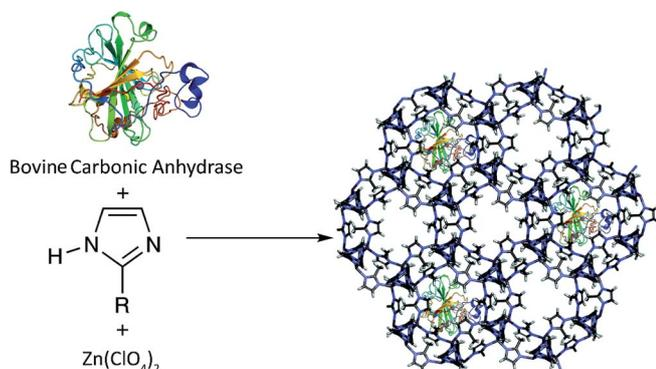
Scheme 2 Schematic representation of the preparation of the BCA-ZIF-8 biocomposite.
