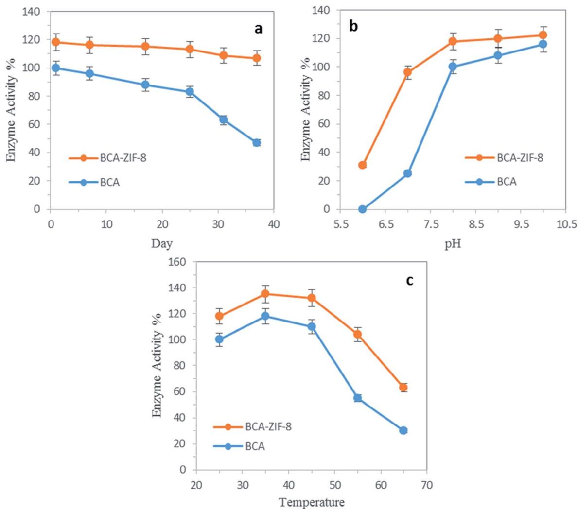
Fig. 7 (a) Storage stability, and (b) effect of pH and (c) temperature on the enzyme activity.
