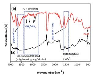
Fig. 16 Fourier transform infrared (FTIR) spectrum of bio-magnetic membrane capsules (BMMCs) (a) before and (b) after the sorption of cationic malachite green (MG) dye.
