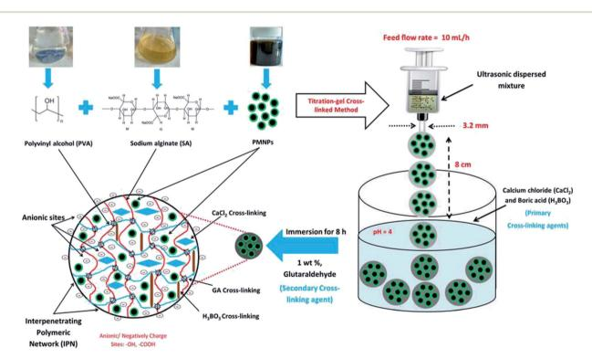
Fig. 1 A schematic diagram of bio-magnetic membrane capsule (BMMC) fabrication by the encapsulation of phytogenic magnetic nanoparticles (PMNPs). (Reproduced from Ali et al.<sup>24</sup> Copyright@2019, with permission from Elsevier Ltd.)
