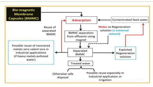
Fig. 18 Proposed conceptual treatment model using bio-magnetic membrane capsules (BMMCs) based on zero-effluent discharge for water/ wastewater containing cationic toxic dyes and heavy metal ions.
