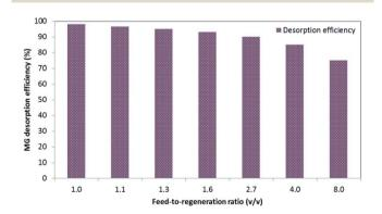
Fig. 14 Effect of different feed-to-regeneration ratios (v/v) on the desorption efficiency of malachite green (MG) dye (water as regeneration solution; adsorbent dosage = 0.02 g L<sup>-1</sup>, MG initial concentration ( $C_o$ ) = 25 mg L<sup>-1</sup>; replication = 3; standard deviation:  $\pm$  1.59).
