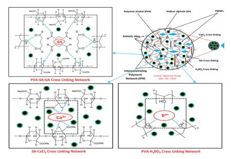
Fig. 3 Conceptual possible cross-linking networks of SA-CaCl<sub>2</sub>, PVA-H<sub>3</sub>BO<sub>3</sub> and PVA-SA-GA during the fabrication of bio-magnetic membrane capsules (BMMCs). (Reproduced from Ali et al.<sup>24</sup> Copyright@2019, with permission from Elsevier Ltd.)
