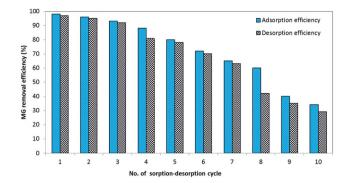
Fig. 15 Study of the stability and reusability of BMMCs for consecutive sorption–desorption cycles of malachite green (MG) dye (15 mL of water as regeneration solution; adsorbent dosage = 0.02 g L<sup>-1</sup>, MG initial concentration ( $C_0$ ) = 25 mg L<sup>-1</sup>; replication = 3; standard deviation:  $\pm$  3.18).
