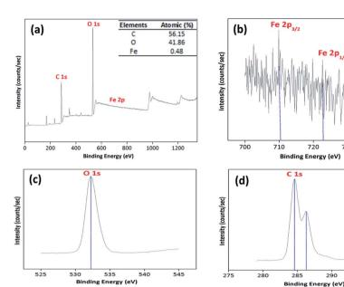
Fig. 6 X-ray photoelectron spectrum (XPS) of (a) bio-magnetic membrane capsules (inset table shows the atomic percentages of the elements); (b) high resolution XPS spectrum of Fe 2p; (c) high resolution XPS spectrum of O 1s; (d) high resolution XPS spectrum of C 1s
