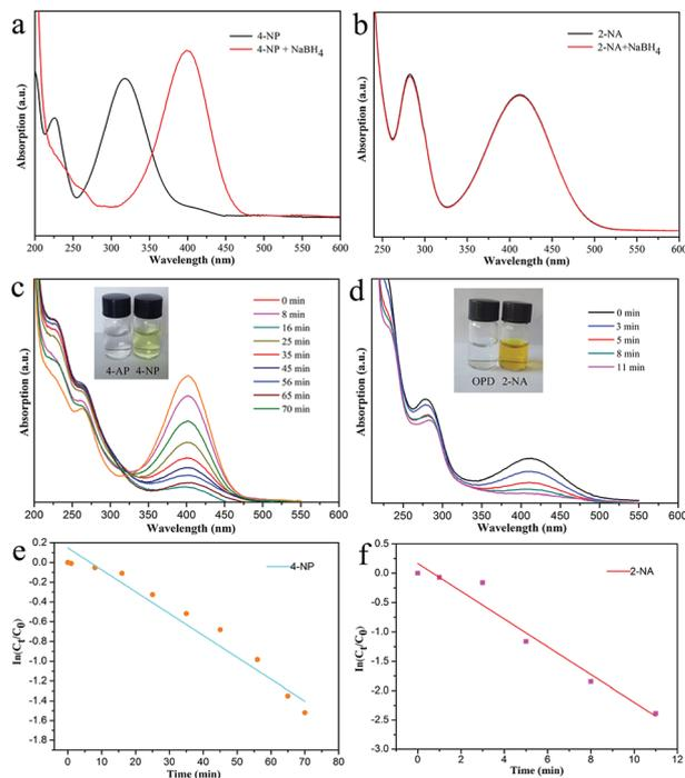
Fig. 7 The spectra of 4-NP and 2-NA with the addition of  $\text{NaBH}_4$  (a and b). Curves of the catalytic reduction of 4-NP (c) and 2-NA (d). Plots of  $\ln(C_t/C_0)$  versus time for 4-NP (e) and 2-NA (f). Pictures (insets in (c) and (d)) represent the solutions before/after the catalytic reaction.
