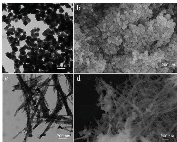
Fig. 2 TEM and SEM images of the prepared Fe<sub>3</sub>O<sub>4</sub> nanoparticles (a and b) and Fe<sub>3</sub>O<sub>4</sub>-Ag nanocomposite (c and d).
