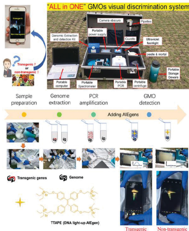
Scheme 1 Scheme for visual discrimination of transgenic and non-transgenic food using DNA-binding AIEgens and a brief introduction of the "ALL in ONE" GMO portable detection system. The portable detection system consisted of the following parts: genomic extraction and detection kit (genomic extraction reagents, mini-column, PCR primers, AIEgens, etc. ); portable power supply; camera obscura (for visual detection); cuvette; pipettes; ultraviolet flashlight (for visual detection); mortar and pestle (for sample preparation); portable storage dewars (for sample preparation); portable centrifuge (for sample preparation); portable PCR device (for genomic sequence replication and amplification); portable spectrometer (for wavelength detection); portable computer (for data acquiring and analysis).
