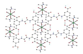
Fig. 8 Schematic illustration of the structure of the Ca-MOF. Several H atoms have been removed for clarity. Color code: Ca, green; C, grey; O, red; N, blue; and H, cyan. Reproduced from ref. 78b with permission from the Royal Society of Chemistry.
