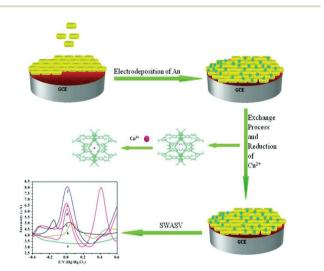
Fig. 5 Schematic representation of the preparation process of the Au/  $Me_2NH_2@MOF-1/GCE$  and the procedures for determination of copper (II) via the cation exchange and nano-particle synergy effect enhanced electrochemical signal. Reproduced from ref. 70 with permission from the Royal Society of Chemistry.
