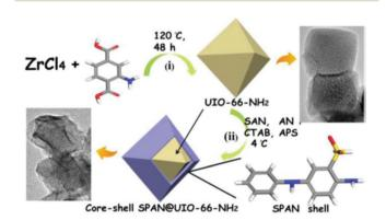
Fig. 4 Schematic representation of the synthetic route of UiO-NH<sub>2</sub>, core-shell SPAN@UIO-66-NH2 and core-shell SPAN@UIO-66-NH2. Reprinted from ref. 69 with permission from The Electrochemical
