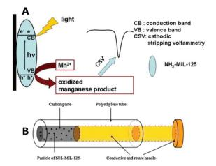
Fig. 6 (A) The photooxidation procedure of Mn<sup>2+</sup> at the NH<sub>2</sub>-MIL-125-Ti/CPE and its determination by CSV. (B) Schematic illustration of the structure of the NH2-MIL-125(Ti) modified carbon paste electrode. Reprinted from ref. 72d with permission from Elsevier.
