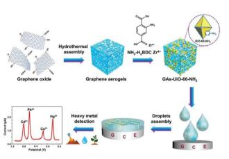
Fig. 7 Synthesis of the GAs-UiO-66-NH<sub>2</sub> composite via the in situ growth of the UiO-66-NH2 crystal on the GAs Matrix and the determination of heavy metal ions with the modified electrode. Reprinted from ref. 74 with permission from American Chemical Society.
