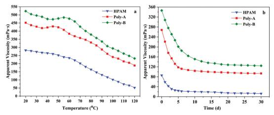
Fig. 7 (a) Temperature resistance and (b) aging resistance of the copolymers.
