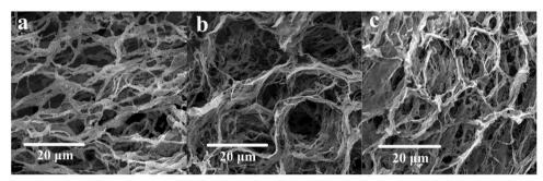
Fig. 3 SEM analysis of the copolymer in deionized water: (a) HPAM, magnified 2000 times; (b) Poly-A, magnified 2000 times; (c) Poly-B, magnified 2000 times (copolymer concentration, 2000 mg  $L^{-1}$ ).
