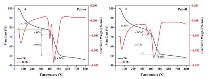
Fig. 4 TG-DTG curves: (a) Poly-A, (b) Poly-B.
