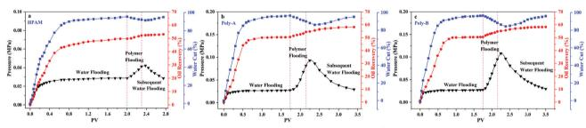
Fig. 11 Core flooding experiments of polymer flooding (copolymer concentration, 2000 mg L<sup>-1</sup>; 70 °C)
