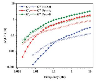
Fig. 9 Viscoelastic behavior of copolymers
