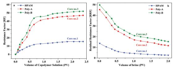
Fig. 10 Flow behavior of copolymer solutions in porous media (copolymer concentration, 2000 mg L<sup>-1</sup>; 70 °C).
