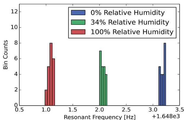
Fig. 5 Resonant frequency of a cantilever is shown for relative humidity values of 0, 34, and 100 percent (cantilever dimensions are: 3 mm long, 100  $\mu\text{m}$  wide, 64  $\mu\text{m}$  high, and a carbon infiltration time of 6 minutes). This histogram shows observations taken while humidity values were sequentially changed in a randomized order. Shifts on the order of 1 Hz were seen on top of a base resonant frequency of 1.65 kHz.
