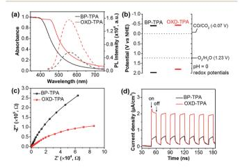
Fig. 2 (a) UV/vis diffuse reflectance spectra (solid line) and photoluminescence (PL) spectra (dashed lines;  $\lambda_{\rm ex}=380$  nm) of BP-TPA and OXD-TPA in the solid state. (b) Energy levels of BP-TPA and OXD-TPA relative to the potentials of CO $_2$  reduction to CO and water oxidation, respectively, vs. the NHE at pH = 0. (c) EIS Nyquist plots and (d) periodic transient photocurrent response of polymer electrodes in 0.5 M Na $_2$ SO $_4$  aqueous solution.
