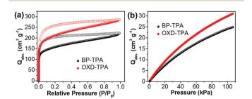
Fig. 1 (a) N<sub>2</sub> sorption isotherm curves of the polymers obtained at 77 K. (b) CO<sub>2</sub> adsorption isotherm curves of the polymers at 298 K.
