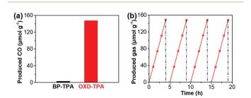
Fig. 3 (a) CO production from the photocatalytic  $CO_2$  reduction over BP-TPA and OXD-TPA after 4 h irradiation (>420 nm). Reaction conditions: 15 mg polymer,  $CO_2$  (1.0 atm), water vapor, room temperature. (b) Time course of photocatalytic  $CO_2$  reduction over OXD-TPA.
