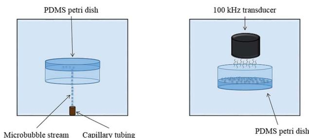
**Fig. 1** Design apparatus for controlled cavitation simulation on PDMS films. MBs are initially collected on PDMS films when the Petri dish is directed downward. The Petri dish is then rotated 180° and exposed to an ultrasound transducer that induces dramatic MB oscillation, resulting in cavitation.
