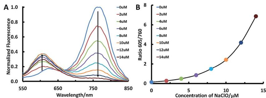
Fig. 1 (A) Emission spectra of **C1O1** (5  $\mu\text{M}$ ) upon treatment with various concentrations of NaClO (0–14  $\mu\text{M}$ ); (B) fluorescence ratio ( $I_{605}/I_{760}$ ) of **C1O1** (5  $\mu\text{M}$ ) upon treatment with various concentrations of NaClO (0–14  $\mu\text{M}$ ).
