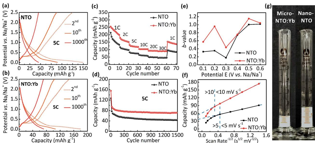
Fig. 2 The 2<sup>nd</sup>, 10<sup>th</sup>, and 1000<sup>th</sup> charge/discharge curves of (a) NTO and (b) NTO:Yb. (c) The rate and (d) cycle performance of NTO and NTO:Yb in a half cell. (e)  $b$ -values for NTO and NTO:Yb as a function of potential for anodic sweeps ( $\text{Na}^+$  insertion). (f) Capacity versus  $\nu^{-1/2}$  allows for the separation of diffusion-controlled capacity from capacitive-controlled capacity. (g) The comparison of tap densities of nano-NTO and micro-NTO:Yb.
