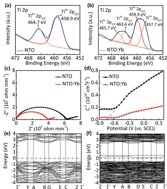
Fig. 3 The Ti 2p XPS spectra of (a) NTO and (b) NTO:Yb. (c) EIS at room temperature of the pellets made from NTO and NTO:Yb for the bulk conductivity measurement. (d) The Mott–Schottky plots of NTO and NTO:Yb at the frequency of 500 Hz. The calculated band structure in the irreducible Brillouin zone of (e) NTO and (f) NTO:Yb.
