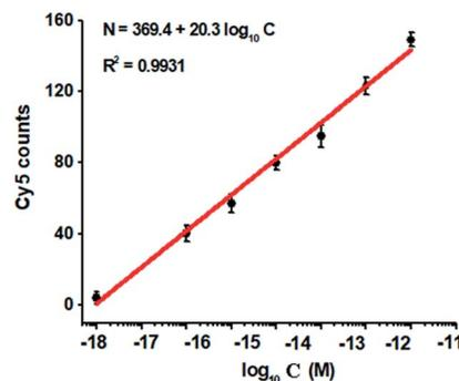
Fig. 4 Variance of Cy5 counts with different-concentration methylated DNA. The Cy5 counts exhibit a linear correlation with the logarithm of methylated DNA concentration in the range from  $1 \times 10^{-18}$  to  $1 \times 10^{-11}$  M. The concentration of each DNA probes X, Y, X' and Y' is  $1.0 \times 10^{-6}$  M. The concentration of 605QD is 8.3 nM. Error bars show the standard deviation of three experiments.
