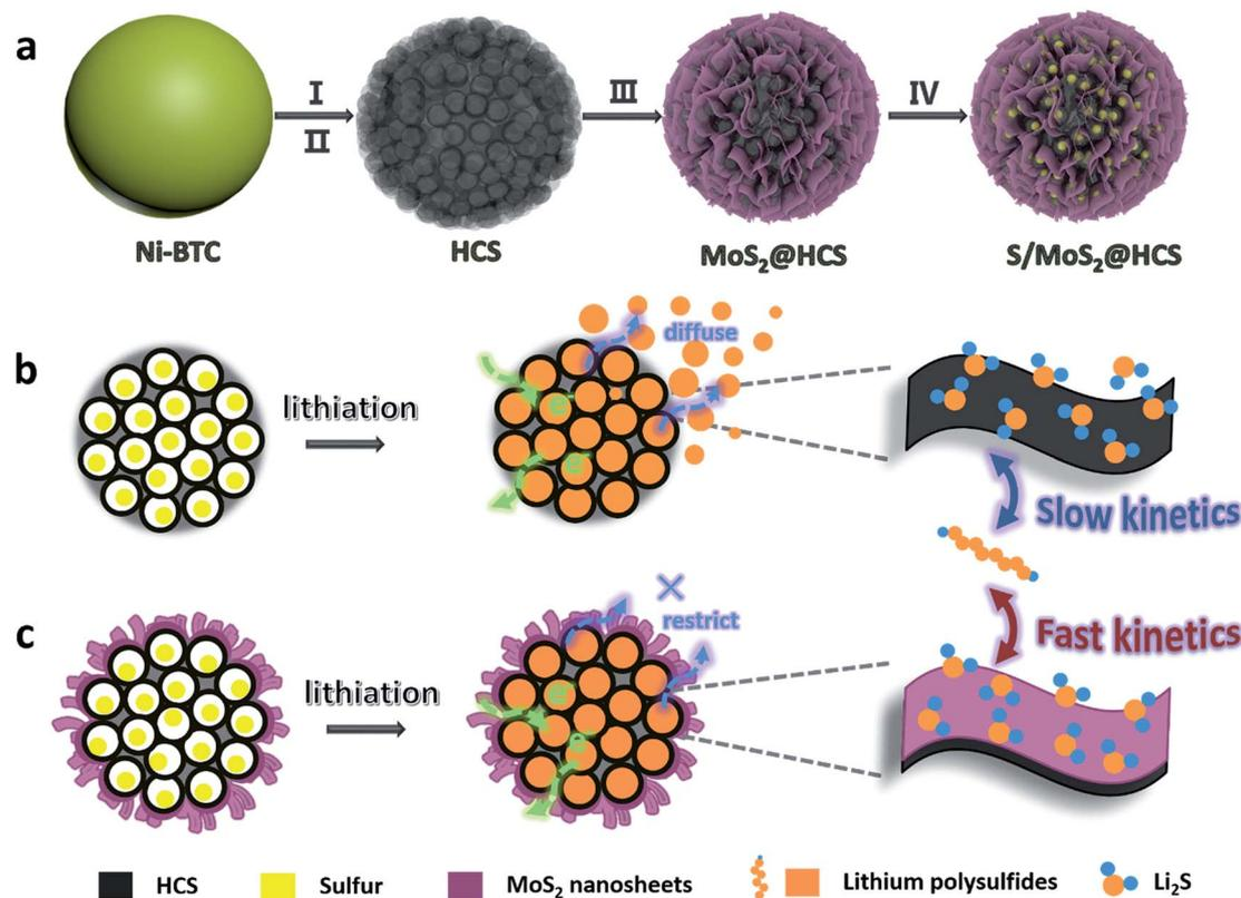
**Scheme 1** (a) Illustration of the synthesis of the S/MoS<sub>2</sub>@HCS composite. (b and c) Illustrations of the advantages of the S/MoS<sub>2</sub>@HCS composite over the S/HCS composite during lithiation.
