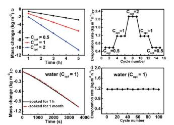
Fig. 3 Durability and stability of the evaporator. (a) The evaporation mass changes of water under different  $C_{\rm opt}$  within 5 hours. (b) The evaporation cycle performance of the evaporator under different solar concentrations. (c) Evaporation rate curves of the evaporator soaked in water after 1 h and 1 month. (d) The evaporation cycle performance of the evaporator in water over 100 cycles, with each cycle sustained for 1 h
