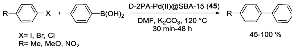
Scheme 59 Reactivity of D-2PA-Pd(II)@SBA-15 (45) for Suzuki-coupling reaction.
