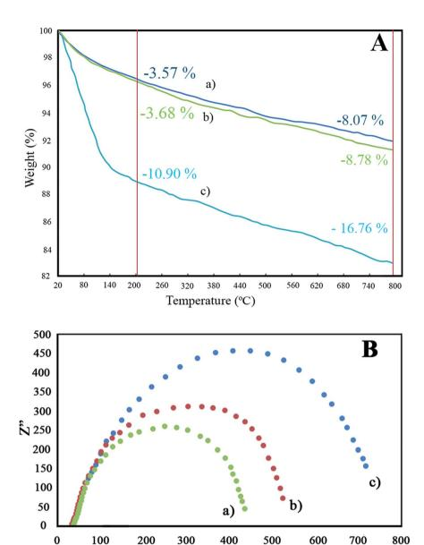
Fig. 7 (A) TGA patterns of (a) Ti, (b) ZnTi, and (c) GZnTi; (B) EIS spectra of (a) Ti, (b) ZnTi, and (c) GZnTi catalysts under visible light irradiation.
