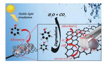
Fig. 12 Tentative photocatalytic Ph-degradation mechanism under visible light irradiation using GZnTi.
