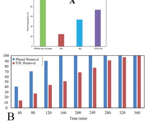
Fig. 10 (A) Ph-degradation efficiency in the presence of different radical scavengers (IPA, BZQ, Na<sub>2</sub>-EDTA); (B) comparison of phenol removal and TOC removal at pH: 4, catalyst dosage:  $0.6 \text{ g L}^{-1}$ , and phenol concentration: 60 ppm.
