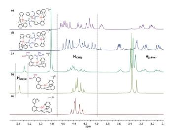
Fig. 2 Comparison of the  $^{1}$ H-NMR signals for the compounds 1, 4, 5-L-Phe, 1-L-Phe and 2-L-Phe in  $D_{3}$ -acetonitrile. In this region acetal (5.4 to 5.2 ppm), CH<sub>2</sub> pycolil (4.6 to 3.9 ppm) and amino acid (3.8 to 2.7 ppm) proton signals are present. The counteranions are perchlorate.
