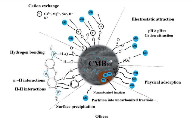
Fig. 10 Interaction mechanisms in the biochar-MB system.
