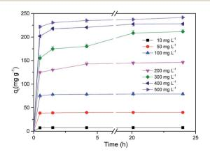
Fig. 5 The effect of contact time on the adsorption capacity at different initial MB concentrations ( $W = 0.025 \, \text{g}$ ,  $V = 20 \, \text{mL}$ ,  $T = 25 \, ^{\circ}\text{C}$ ).
