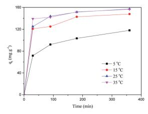
Fig. 7 The effect of contact time on the adsorption capacity at different temperatures ( $W=0.025~{\rm g},~V=20~{\rm mL}$ ).
