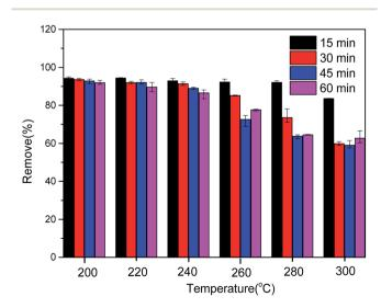
Fig. 3 Effect of torrefaction temperature and torrefaction time of CMB on removal rate. ( $C_0 = 100 \text{ mg L}^{-1}$ , W = 0.01 g, V = 20 mL, t = 80 min,  $T = 25 \,^{\circ}\text{C}$ ).
