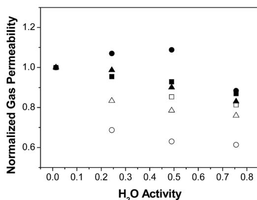
Fig. 2 Normalised gas permeability  $P/P_{dry}$  through the zeolite A/PTMSP MMM, (full symbols) PTMSP membranes (void symbols): N<sub>2</sub> (triangles), CH<sub>4</sub> (squares), CO<sub>2</sub> (circles).
