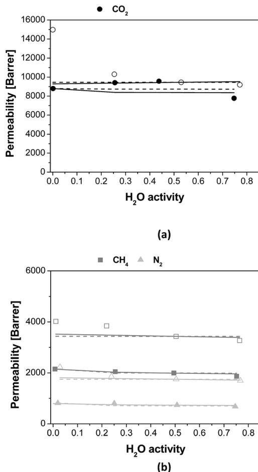
Fig. 7 Permeability of (a) CO<sub>2</sub> (black circles) and (b) N<sub>2</sub> (light grey triangles) and CH<sub>4</sub> (grey squares) as function of water activity for the PTMSP membrane (void symbols) and the zeolite A/PTMSP MMM (full symbols). Dashed lines correspond to the diffusivity-based model and continuous lines to the (diffusivity + solubility)-based model.
