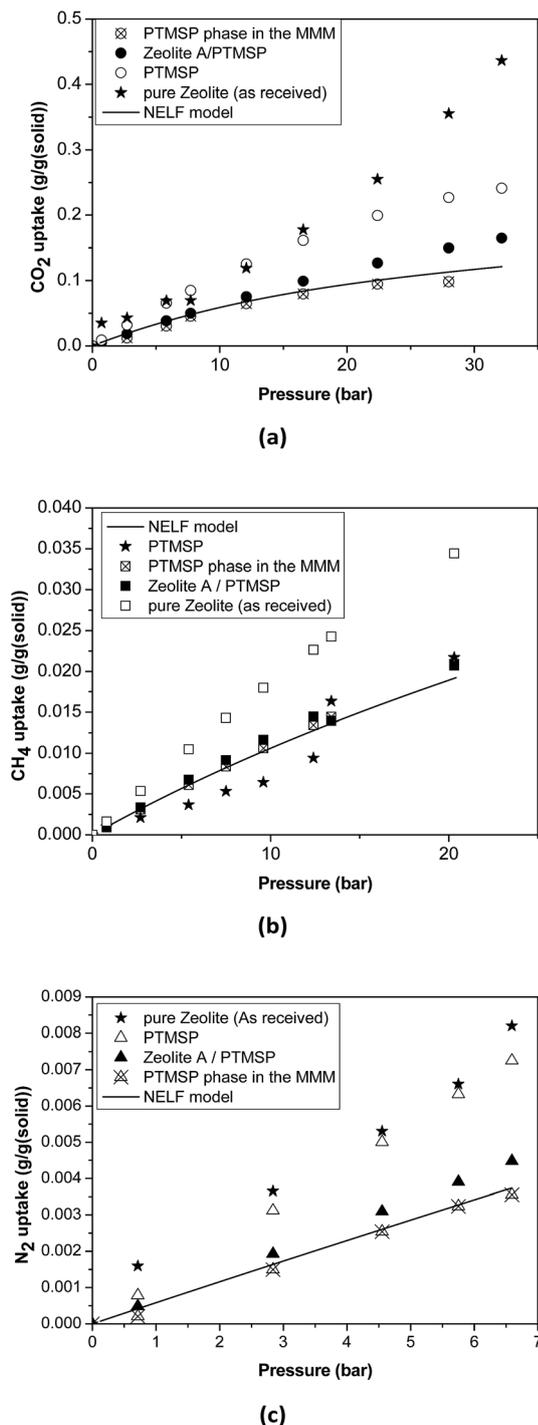
Fig. 4 Sorption isotherms in the pure zeolite, pure PTMSP, zeolite A/PTMSP MMM and the PTMSP phase in the MMM. The solid line represents the adjustment with the NELF model.
