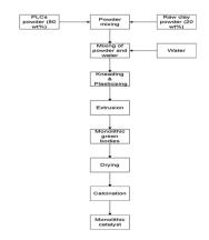
Fig. 2 Schematic representation of extrusion process.
