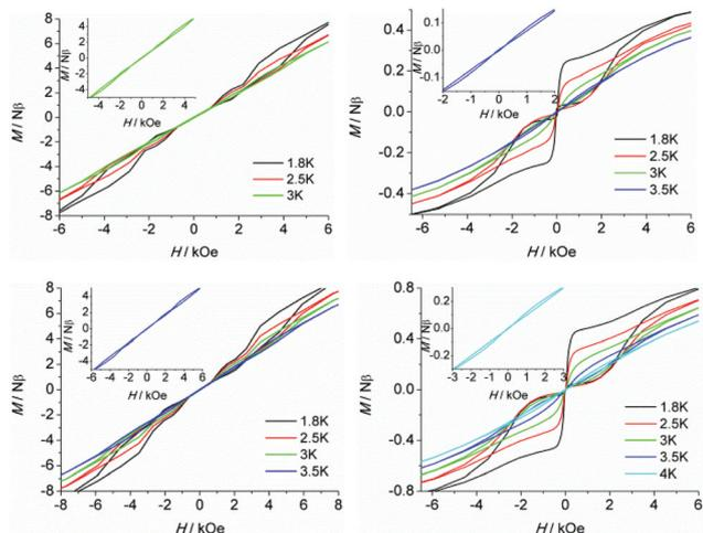
**Fig. 12** Field dependence of the normalized magnetization of samples **2** (top left), **2b** (top right), **de1** (bottom left) and **de1b** (bottom right) between 1.8 and 4 K at a sweep rate of 200 Oe s<sup>-1</sup>. Inset: *M* versus *H* plots for each at the highest temperature.
