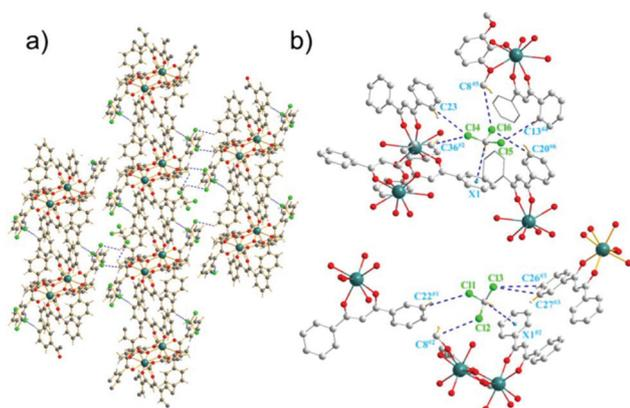
**Fig. 2** (a) Crystal packing of **1** along the  $a$ -axis. Dy, dark blue; O, red; C, grey; H, white; Cl, green. (b) Views showing the C–H... $\pi$  interactions and intermolecular H–C...Cl interactions among the crystallographically equivalent Dy–DMOP units of **1** (hydrogen atoms have been omitted for clarity; symmetry codes: #1:  $1 - x, 1 - y, z$ ; #2:  $1 - x, 1 - y, 1 - z$ ; #3:  $x - 1, y, z$ ; #4:  $1 - x, -y, -z$ ; #5:  $x, y, z - 1$ ; #6:  $1 + x, y, z$ ).
