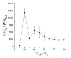
Fig. 5 ILs with high distribution of Cu<sup>2+</sup> into the IL phase;  $[C_4C_1im][OAc].$
