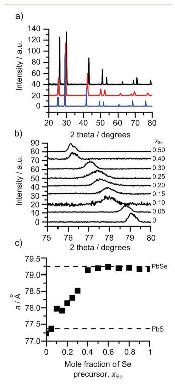
Fig. 3 XRD analysis of the  $PbS_xSe_{1-x}$  films. (a) XRD patterns from  $x_{Se}=0$  (black),  $x_{Se}=0.25$  (red) and  $x_{Se}=0.5$  (blue). (b) XRD patterns of the 422 reflection from  $x_{Se}=0$  to 0.5. (c) Shows a plot of mole fraction against the position of the 422 reflection as compared to the values from the reference patterns (PbSe ICDD 00-006-0354 and PbS ICDD 00-005-0592) shown with dashed lines.
