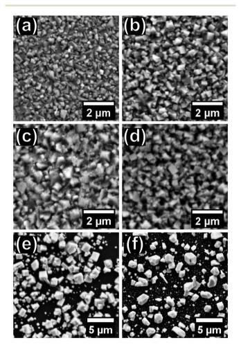
Fig. 5 Scanning electron micrographs of  $PbS_xSe_{1-x}$  films produced from  $x_{\text{(Se precursor)}} = 0$ , 0.1, 0.2, 0.3, 0.4, 0.5 and 0.6 represented by (a) to (f) respectively.
