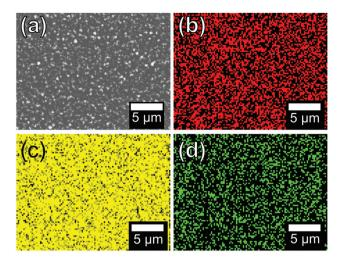
**Fig. 6** An SEM image for the alloyed films produced using  $x_{(Se\ precursor)} = 0.3$  (a) and the corresponding EDX maps for Pb, S and Se (b), (c) and (d) respectively.
