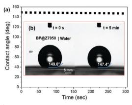
Fig. 4 Contact angle measurements on a PVDF membrane with BP immobilized at the surface. (a) Plot of contact angle (°) over time for a drop of deionized water on the BP supported by PVDF membrane. (b) Optical images (CCD camera) of the contact angle of a deionised water droplet on the BP-coated membrane at t=0 and 5 min.
