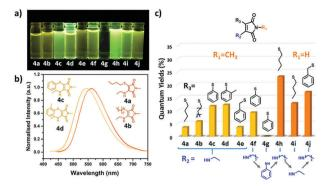
Fig. 2 (a) Solution of **ATMs** under UV light (365 nm); (b) emission spectra of different alkyl thiol (**4a–b**) and thiophenol (**4c–d**) aminomaleimides (recorded at 10  $\mu$ M in diethyl ether); (c) fluorescence quantum yields of studied **ATMs** in diethyl ether.
