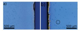
**Fig. 2** Optical microscopy images of the SiC surface grown with  $T=1550~^{\circ}\text{C}$  and different C precursors. (a) 10 cm from the inlet using  $\text{C}_3\text{H}_8$  showing a rough surface indicative of no growth and no onset of epitaxial growth, (b) 3 cm from the inlet using CH<sub>4</sub> showing a smooth surface with a triangular surface defect (circled) indicative of epitaxial
