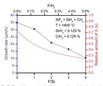
Fig. 7 The relative amount of surface vacancies available for chemisorption of C-bearing growth species and the growth rate obtained for various F/Si or  $F/H_2$  ratios.
