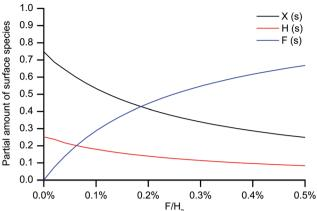
**Fig. 6** Equilibrium composition of the surface species at different  $F/H_2$  ratios from quantum-chemical modeling. H (s) denotes hydrogen termination, X (s) denotes surface vacancy, F (s) denotes fluorine termination.
