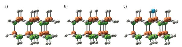
Fig. 5 The SiC cluster models used in this study of (a) the completely hydrogen-terminated surface – H (s), (b) the cluster with a dangling bond – X (s) and (c) the single fluorine-terminated structure - F (s).
