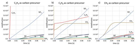
Concentrations of main gas phase species at T = 1550 °C from kinetic simulations when the carbon precursor is (a)  $C_2H_4$ , (b)  $C_3H_8$ , (c)  $CH_4$ .
