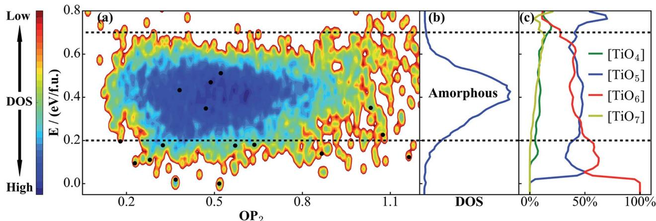
Fig. 5 (a) PES contour plot for  $TiO_2$  distinct minima sampled from the SSW-NN global search. (b) Density of states (DOS) plot for  $TiO_2$  phases in (a), showing that amorphous structures appear in the 0.2–0.7 eV f.u.<sup>-1</sup> window. (c) The percentage of differently coordinated Ti for  $TiO_2$  structures.  $[TiO_5]$  and  $[TiO_6]$  are the main structural features for amorphous structures. Also see the Fig. 2 caption for the meaning of the black dots.
