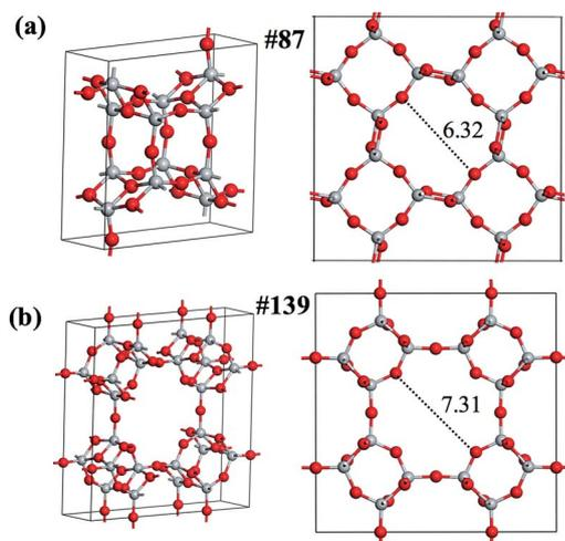
Fig. 6 Two new porous  $TiO_2$  phases identified from the SSW-NN global search. (a) Phase-87; (b) phase-139. The Bravais lattices are shown on the left and the pore geometries with the pore size labeled are shown on the right.
