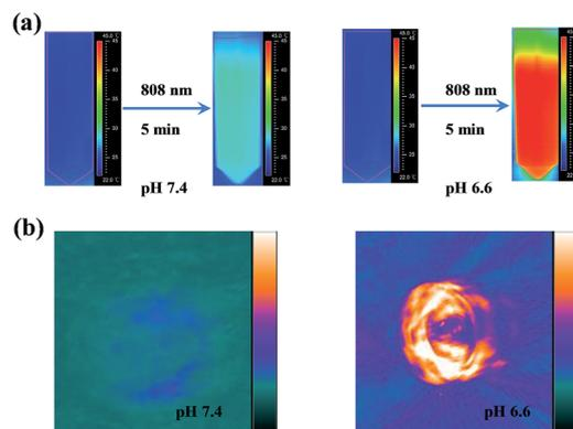
**Fig. 2** *In vitro* photothermal imaging and PA imaging. (a) Photothermal images of the gold nanomachines at pH 7.4 (left) or 6.6 (right) with 5 min of irradiation were captured. (b) An obvious PA signal appeared when the gold nanomachines were incubated at pH 6.6 (right) compared to that at pH 7.4 (left).
