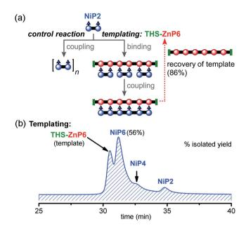
Fig. 9 Reaction design and outcome of linear tetramer templating for the synthesis of NiP6 from NiP2 using THS-ZnP6 as a template. (a) Reaction scheme. (b) GPC traces (detection at 646 nm, THF) of the linear templating reaction product mixture with the template THS-ZnP6. Products were identified by MLALDI-ToF and <sup>1</sup>H-NMR for NiP6.
