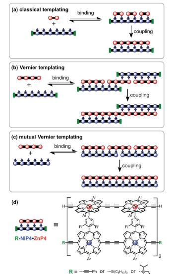
Fig. 1 Linear template-directed syntheses of monodisperse linear porphyrin oligomers. (a) Classical template-directed synthesis. (b) Vernier templating synthesis. (c) Mutual Vernier templating: both strands couple. (d) Key to molecular design.
