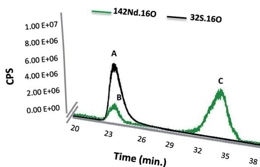
Fig. 3 Chromatograms obtained by SEC-ICP-MS for labelled SA in HSA with Nd-DOTA-KE. Monitored isotopes were  $^{142}\text{Nd}$  and  $^{32}\text{S}$  where both were measured with the oxygen reaction mode. Monitored  $^{32}\text{S}^{16}\text{O}$  represented in peak A is related to the total HSA in the sample, where monitored  $^{142}\text{Nd}^{16}\text{O}$  represented in peak B is related to the labelled HSA with Nd-DOTA-KE, and finally peak C represents the excess of the labelling reagent.
