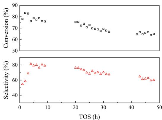
Fig. 6 Catalyst stability of EtOH/ult-0 h-500 within 48 h. Temperature 350 °C, WHSV = 2.5 h<sup>-1</sup>, LA feedstock: 20 wt% in water, carrier gas N<sub>2</sub>: 30 mL min<sup>-1</sup>.
