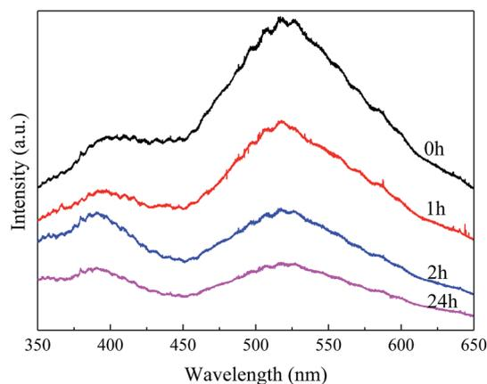
Fig. 3 Photoluminescence (PL) spectra of BaSO<sub>4</sub> catalysts with different aging time.
