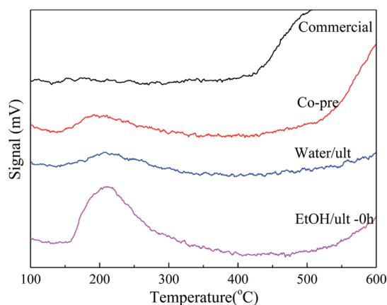
Fig. 4 NH<sub>3</sub>-TPD profiles of BaSO<sub>4</sub> catalysts prepared with different methods.
