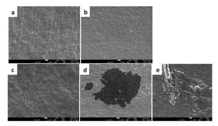
Fig. 11 Scanning Electron Micrographs (SEM) of: (a) pristine LDPE-AEM (100 kGy); (b) pristine ETFE-AEM (30 kGy); (c) LDPE-AEM (100 kGy) degraded in aqueous NaOH (1 mol dm $^{-3}$ ) for 7 d at 80 °C; (d and e) similarly degraded ETFE-AEM (30 kGy). The white scale bars = 1  $\mu m$ .
