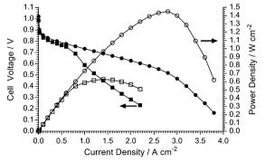
Fig. 13 The AEMFC performances at 80 °C of the LDPE-AEM (100 kGy) with  $O_2$  ( $\bullet$ , $\bigcirc$ ) and  $CO_2$ -free air ( $\blacksquare$ , $\square$ ) supplies ay the cathode: PtRu/C (50% wt Pt and 25% wt Ru) anodes and Pt/C (40% wt) cathodes (all  $0.4 \text{ mg}_{Pt} \text{ cm}^{-2}$  loadings). The 1.0 SLPM (RH = 100%) cathode and anode (H<sub>2</sub>) gas supplies were not pressurised.
