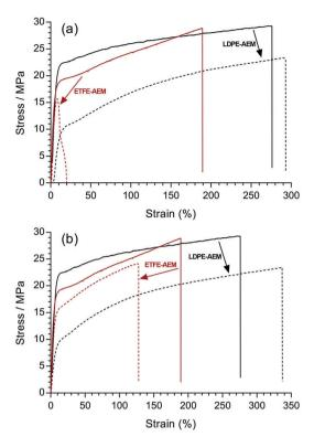
Fig. 10 (a) The tensile stress-strain curves before (solid) and after (dashed) the LDPE-AEM (100 kGy) (black) and the ETFE-AEM (30 kGy) (red) were aged in aqueous NaOH (1 mol dm $^{-3}$ ) for 7 d at 80 °C. (b) The corresponding data where the RG-AEMs were aged in alkali at 60 °C.
