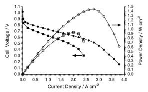
Fig. 14 The H<sub>2</sub>/O<sub>2</sub> AEMFC performances at 80 °C of the LDPE-AEM (100 kGy) with Pt/C (0.4 mg<sub>Pt</sub> cm<sup>-2</sup>) ( $\bullet$ , $\bigcirc$ ) and Ag/C (0.8 mg cm<sup>-2</sup>) (  $\blacksquare$  ,  $\square$  ) cathodes: PtRu/C (50% wt Pt and 25% wt Ru) anodes (0.4  $mg_{Pt}\,cm^{-2}$ loading). The 1.0 SLPM (RH = 100%) gas supplies were not pressurised.
