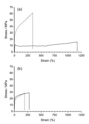
**Fig. 7** Tensile stress–strain curves for: (a) the pristine LDPE (solid) and ETFE (dashed) precursor films; (b) LDPE-AEM (100 kGy) (solid) and ETFE-AEM (30 kGy) (dashed), where the RG-AEMs were in the Cl<sup>-</sup> anion forms (dehydrated). The x- and y-axes were left at the same scale to demonstrate the change in tensile properties after grafting and amination (the expanded data is presented in Fig. S7 in the ESI†).
