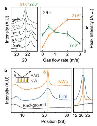
Fig. 2 (a) (left) XRD patterns of nanowire-filled templates crystallised at various assisted gas-flow rates. (right) Based on the normalised XRD patterns, the average intensity of the peak at 21.6° and 22.6° is plotted as a function of assisted-gas flow rate. (b) XRD patterns of a nanowire-filled template (orange), melt-quenched film (blue), and silicon background (grey). The right image shows the magnification of the  $\delta'$ -phase range.
