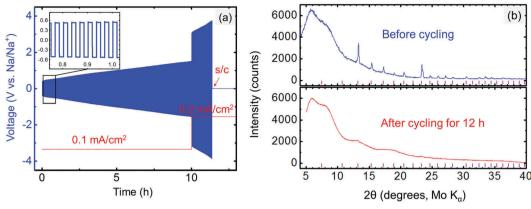
Fig. 8 (a) Electrochemical cycle for  $Na|Na_3PSe_4|Na$  symmetric cell; a short circuit (s/c) occurred after cycling for 11.4 h. (b) XRD results for  $Na_3PSe_4$  before and after cycling for 12 h (1 min per cycle); the tick marks indicate  $Na_3PSe_4$  peaks.
