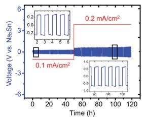
Fig. 10 Electrochemical cycling of  $Na_2Sn|Na_3PS_4|Na_2Sn$  symmetric cell (60 min per charge and discharge). The insets present zoomed-in voltage profiles during cycling from 2–6 h and 96–100 h.
