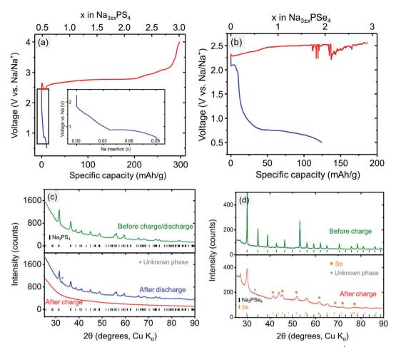
Fig. 3 Electrochemical cycling of the  $Na_3PX_4$  (mixed with carbon) cathode composite at constant current (2.604 mA  $g^{-1}$  for  $Na_3PS_4$  and 2.404 mA  $g^{-1}$  for  $Na_3PS_4$ , showing the stability window of (a)  $Na_3PS_4$  and (b)  $Na_3PS_4$ . Diffraction patterns of the (c)  $Na_3PS_4$  cathode composite before and after being fully charged/discharged and (d)  $Na_3PS_4$  cathode composite before and after being fully charged.
