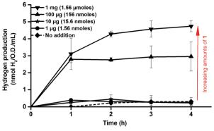
Fig. 2 In vivo H<sub>2</sub> production of E. coli cultures in glucose enriched LB media observed following in vivo artificial activation of apo-HydA1 in early log-phase E. coli cultures (O.D. = 0.20  $\pm$  0.02) using varying amounts of complex 1. H<sub>2</sub> measured by sampling the headspace gas every hour. All data points represent means of at least two independent repeats with duplicate samples from each culture, error bars  $\pm$  S.D.
