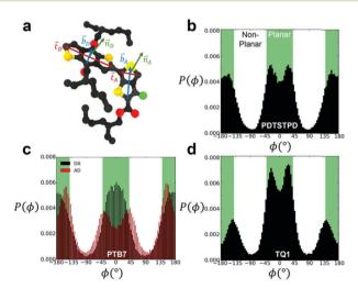
Fig. 2 Inter-ring dihedral distributions. (a) Diagram showing definitions of basis sets defining ring orientations for PTB7 monomer. Dihedral distributions,  $P(\phi)$ , obtained from simulations at 600 K and 1 atm for (b) PDTSTPD (c) PTB7 (d) TQ1. The syn conformations shown in Fig. 1 represent the planar arrangement that results from  $\phi$  = 0°
