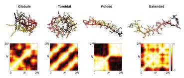
Fig. 6 Conformational classes. Representative chains and their associated orientational contact maps illustrating the conformational classes available to single chains and the distinctive patterns used for classifying the chain conformations.
