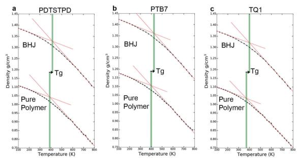
Fig. 5 Thermal properties, density vs. temperature curves showing glass-transitions of polymer: PC71BM bulk heterojunctions (top curves) and pure polymers (bottom curves) for (a) PDTSTPD, (b) PTB7, and (c) TQ1.
