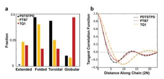
Fig. 7 Characterization of conformational preferences. (a) Chart showing fraction of each conformation present in the self-aggregated morphology for each type of polymer. (b) Tangent correlation function showing a large tendency for folded chains
