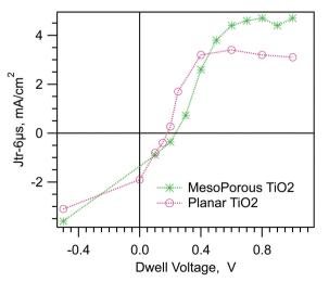
Fig. 2 Results for the SDP experiment on two MAPI cells.  $J_{tr}$ -6 $\mu$ s after a dwell time of 100  $\mu s$  vs. dwell voltage
