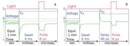
Scheme 2 (a) Time sequence of the Step-Dwell-Probe (SDP) photocurrent transient experiment. (b) Time sequence of the Step-Dwell-Step-Probe (SDSP) photocurrent transient experiment.  $V_d$  is the dwell voltage and  $V_{pr}$  is the probe voltage.
