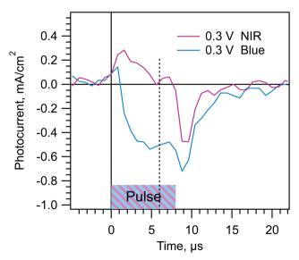
Fig. 5 Effect of blue vs. NIR (735 nm) pulses at  $V_{\rm d}$  and  $t_{\rm d}$  where the photocurrents from regions I and III vs. region II are balanced for the NIR pulse. The peaks at 1  $\mu$ s and 9  $\mu$ s are from the switching of the LED. Data from a m-TiO<sub>2</sub>/MAPI cell with  $t_d$  = 2 ms and  $V_d$  = 0.3 V.
