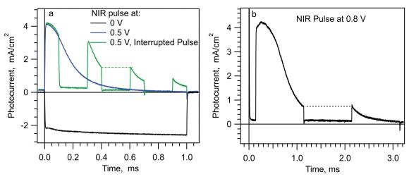
Photocurrent transients from longer light pulses. Transients from the same planar cell shown in Fig. 1 and 2. Pulses from a 735 nm LED
