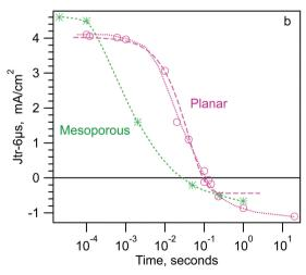
Fig. 3 (a) Photocurrent transients from the SDP experiment for a dwell voltage of 0.8 V and various dwell times. (b)  $J_{tr}$ -6 $\mu$ s vs. dwell time at dwell voltage 0.8 V for the planar and mesoporous cells used in Fig. 1 and 2.
