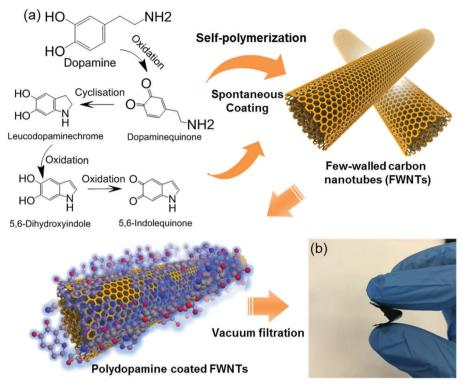
Scheme 2 (a) Oxidative self-polymerization reactions of dopamine in weak alkaline solution and a continuous coating process of polydopamine on the surface of few-walled carbon nanotubes (FWNTs). (b) Digital image of a flexible hybrid film consisting of polydopamine coated FWNTs.
