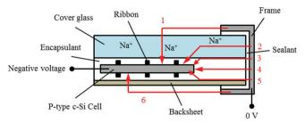
Fig. 2 Cross section of a conventional c-Si PV module constructed with a glass-encapsulant-cell-encapsulant-backsheet package and modelling of the possible leakage current pathways. The solar cells are negatively biased whereas the module frame is grounded. The arrow represents the direction of leakage currents. Positive ions such as sodium ions (Na<sup>+</sup>) drift to the cell when the cells are at negative voltage potential (e.g. through path 1). Adapted from ref. 44.
