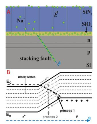
Fig. 6 (A) Schematic drawing of a solar cell cross section and transport of  $\mathrm{Na}^+$  (green dots) through the  $\mathrm{SiN}_{x}$  layer and subsequent diffusion into the stacking faults. (B) The proposed band structure along a Na decorated stacking fault. Reprint from ref. 65. Copyright 2014, Elsevier.
