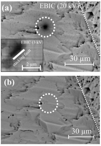
Fig. 25 EBIC measurements (20 kV) at a PID shunt location before (a) and after (b) a thermal recovery process. The PID-s disappeared after recovery The inset in (a) shows the PID-s defect before recovery at la low electron acceleration voltage (3 kV) and hence with an increased lateral resolution. The dotted line represents a grain boundary as guide to the eyes. Reprint from ref. 72. Copyright 2014, Elsevier.
