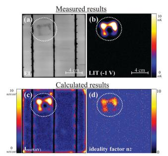
Fig. 22 (a) EL image of a degraded solar cell; (b) DLIT image at -1 V; (c)  $J_{02}$  distribution calculated from DLIT measurements based on the method reported in ref. 128; (d) Ideality factor  $n_2$  distribution, scaled from 2 to 10. Reprint from ref. 63. Copyright 2014, IEEE.
