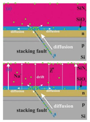
Fig. 27 Schematic diagram of the proposed process for thermal recovery (a) and electrical recovery (b). The green dots represent the Na specie. Na diffuses out of the stacking faults, which leads to power regeneration. The movement of Na is marked by the white arrows. Reproduced from ref. 72. Copyright 2014, Elsevier.
