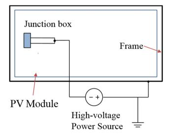
Fig. 12 Schematic diagram of the PID test setup in a climate chamber. The two leads of the PV module are shortened and connected to the negative terminal of a high-voltage power source. The module frame is grounded.
