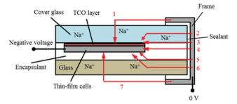
Fig. 3 Cross section of a thin-film PV module with a glass sheet as back cover and modelling of the possible leakage current pathways. The solar cells are negatively biased whereas the module frame is grounded. The arrow represents the direction of leakage currents. Positive ions such as Na+ drift to the cell when the cells are at negative voltage potential (e.g. through paths 1 and 7). Adapted from ref. 22.
