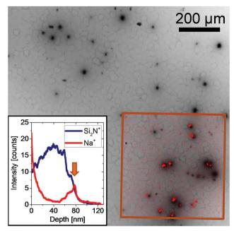
Fig. 4 An EBIC image of a monocrystalline silicon cell region with a high density of PID shunts acquired at an acceleration voltage of 30 kV. The inset shows the distribution of Na at the SiN<sub>x</sub>/Si interface measured by the ToF-SIMS. Reprint from ref. 65. Copyright 2014, Elsevier.
