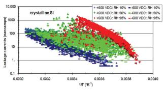
Fig. 16 Leakage current at 600 V DC for mono-crystalline Si modules versus the inverse module temperature in three bands of RH values; the humidity variations are within 2%. Reprint from ref. 115. Permission granted by both the SPIE committee and the author.
