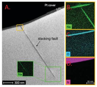
Fig. 5 (A) A bright-field TEM image of a stacking fault representing a single PID-shunt. (B-D) EDX mappings acquired in the STEM mode at the same stacking fault near the interface between Si and SiN<sub>x</sub>. A Na-EDX map of the lower part of the stacking fault is also shown in the inset of A. Reprint from ref. 65. Copyright 2014, Elsevier.
