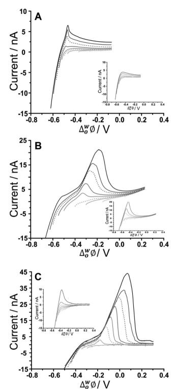
**Fig. 3** AdSV in the presence and absence (inset) of 500  $\mu$ g mL<sup>-1</sup> *U. pinnatifida* fucoidan, in aqueous phase of 10 mM NaOH (pH 12) following adsorption at different potentials. Adsorption time: 60 s, (A) Cell 1, (B) Cell 2, and (C) Cell 3 (Scheme 1). Scan rate: 5 mV s<sup>-1</sup>.
