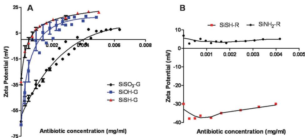
**Fig. 3** Zeta-potential of silica particles as a function of antibiotic concentration. (A) Gentamicin-loaded sulfonate (SiSO<sub>3</sub>-G), unmodified (SiOH-G), and thiol (SiSH-G) modified particles. (B) Rifamycin loaded amino (SiNH<sub>2</sub>-R) and thiol (SiSH-R) modified particles.
