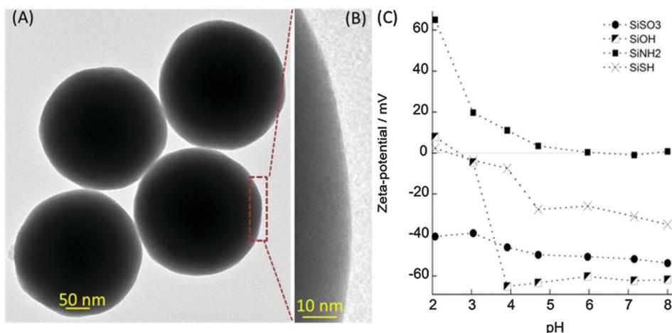
Fig. 1 (A and B) TEM photo of unmodified SiOH particles. (C) Zeta-potential of sulfonate-modified (SiSO<sub>3</sub>), unmodified (SiOH), amino-modified (SiNH<sub>2</sub>) and thiol-modified (SiSH) silica particles at different pH values (10 mM KCl).
