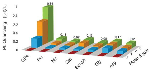
Fig. 4 Selectivity study by fluorescence emission spectrophotometry assessing impact of model analytes on emission intensity of **1** ( $1 \times 10^{-5}$  M;  $\lambda_{\text{ex}} = 340$  nm;  $\lambda_{\text{em}} = 609$  nm; THF; 298 K). DPA: dipicolinic acid; Pic: 2-picolinic acid; Nic: nicotinic acid; Cat: catechol; BenzA: benzoic acid; Gly: glycine; Asp: L-aspartic acid.
