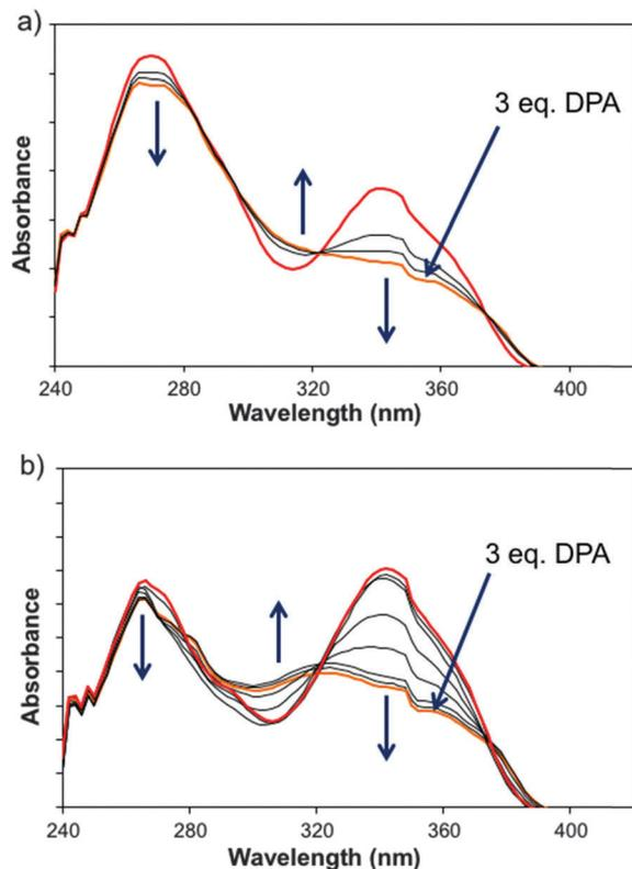
Fig. 2 UV-Vis titration experiments where  $\text{Eu}(\text{Tta})_3\text{Phen}$  ( $1 \times 10^{-5}$  M; THF) is titrated with (a) DPA ( $2 \times 10^{-4}$  M; THF) and (b) DPA ( $2 \times 10^{-4}$  M; THF) in the presence of 2% water and 0.5 equivalents of  $\text{TBA}\cdot\text{H}_2\text{PO}_4$  ( $2 \times 10^{-4}$  M) at 298 K.
