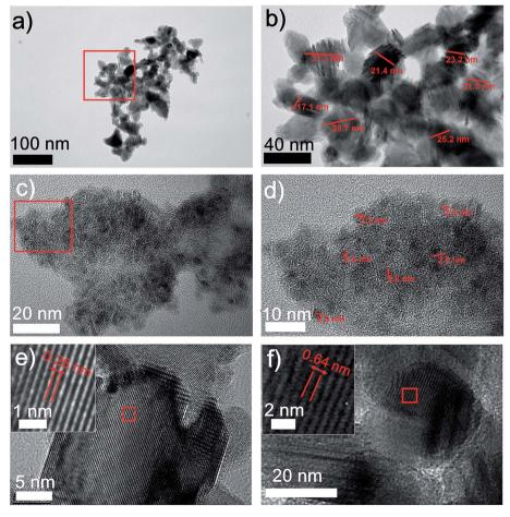
Fig. 2 (a) and (b) TEM images of  $MoS_2$  NPs in the laser-induced  $MoS_2$ /carbon hybrids; (c) and (d) TEM images of  $MoS_2$  QDs in the laser-induced  $MoS_2$ /carbon hybrids; (e) and (f) HRTEM images of  $MoS_2$  NPs in the laser-induced  $MoS_2$ /carbon hybrids. Inset images show their lattice spacings of 0.26 and 0.64 nm, indicating the (200) and (100) planes of  $MoS_2$  NPs.
