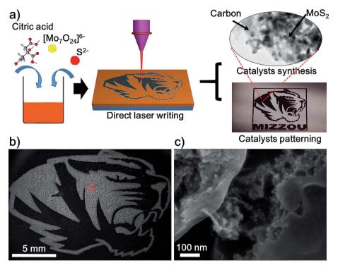
Fig. 1 (a) Scheme of the DLW method in fabricating arbitrary patterns composed of MoS<sub>2</sub>/carbon hybrids. (b) SEM image of a patterned Mizzou tiger logo composed of MoS<sub>2</sub>/carbon hybrids. (c) Magnified SEM image of the selected area indicated in (b).
