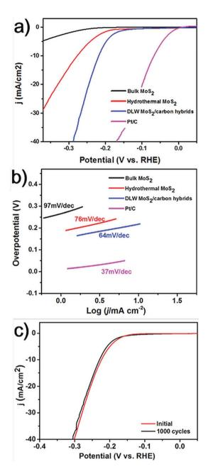
Fig. 4 (a) Polarization curves of Pt/C, bulk MoS<sub>2</sub>, hydrothermal MoS<sub>2</sub>, and laser induced MoS<sub>2</sub>/carbon hybrids. (b) Tafel plots of Pt/C, bulk MoS<sub>2</sub>, hydrothermal MoS<sub>2</sub>, and laser induced MoS<sub>2</sub>/carbon hybrids. (c) Polarization curves of laser induced MoS<sub>2</sub>/carbon hybrids before and after 1000 cycles of CV sweeping.
