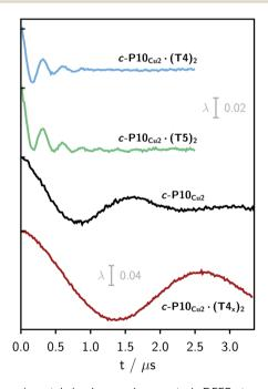
Fig. 6 Experimental background-corrected DEER traces for c- $P10_{Cu2} \cdot (T4)_2$ ,  $c-P10_{Cu2} \cdot (T5)_2$  and  $c-P10_{Cu2}$  (from top to bottom) recorded at 15 K in toluene- $d_8$ . The bottom panel shows the DEER trace of a complex of c-P10<sub>Cu2</sub> with an isomer of T4, referred to as T4<sub>x</sub> as discussed in the main text. The modulation depth scale of 2% refers to the upper three traces, whereas the scale of 4% applies to the bottom trace.
