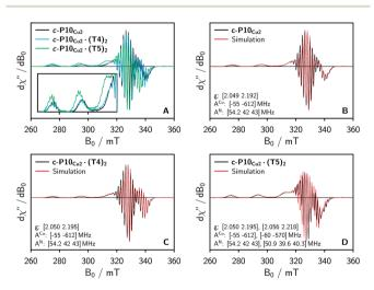
Fig. 3 (A) Comparison of the baseline corrected continuous wave EPR spectra of the investigated samples at 100 K recorded at X-band in frozen toluene- $d_8$ . (B–D) Numerical simulations of the experimental data as explained in the main text. The simulation parameters are indicated in the figure. The relative contribution of the second component in the simulation for  $c\text{-P10}_{\text{Cu2}}\cdot\text{(T5)}_2$  amounts to  $\approx 40\%$ .
