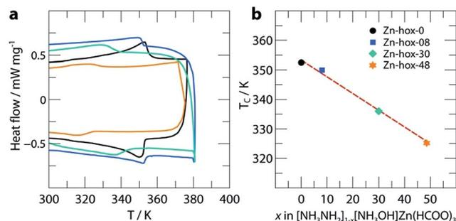
Fig. 2 DSC data (a) and phase transition temperatures (b) as a function of  $x$  in  $[\text{NH}_3\text{NH}_2]_{1-x}[\text{NH}_3\text{OH}]_x\text{Zn}(\text{HCOO})_3$ . The dotted red line acts as a guide for the eye.
