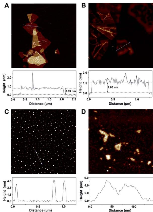
Fig. 2 AFM images and height profiles of (A) bare cGO, (B) MGCB-cGO, (C) antibody molecules, and (D) MGCB-Ab2-cGO on freshly cleaved mica. MGCB-Ab2-cGO exhibits brighter spots with increased heights ( $\sim 5.0$  nm) on its surface.
