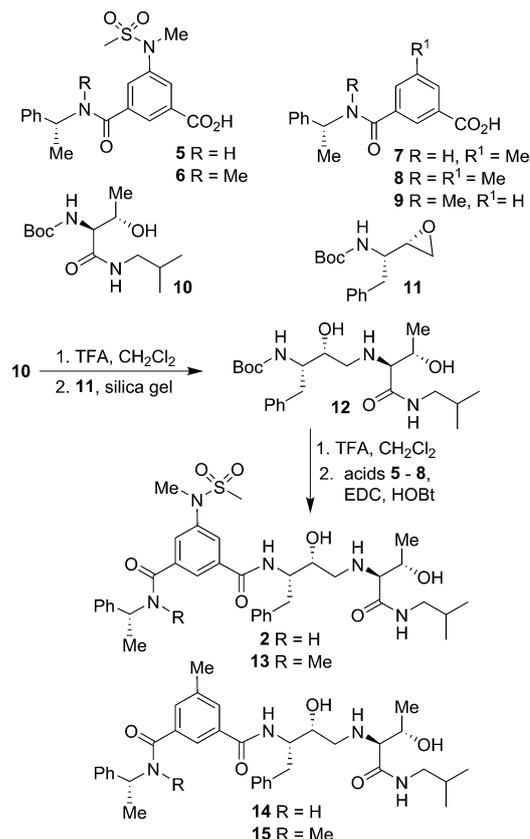
Scheme 1 Synthesis of BACE2 inhibitors **2** and **13**–**15**.
