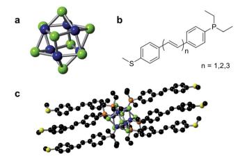
Fig. 1 (a) Structure of the cluster core  $Co_6Se_8$ . (b) Chemical structure of the conducting ligand series Ln (n=1,2,3). (c) Molecular structure of 1 as characterized by single crystal X-ray diffraction. Carbon, black; cobalt, blue; selenium, green; phosphorus, orange; sulfur, yellow.
